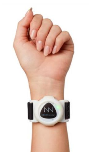
Figure 5: NeuroNode set up on forearm to measure index finger flexion
